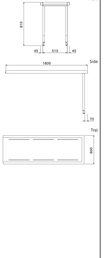
External dimensions, Width:<br/>865304 (BHHLU18)1800 mmExternal dimensions, Depth:<br/>External dimensions, Height:600 mm910 mm910 mmNet weight:18 kg
